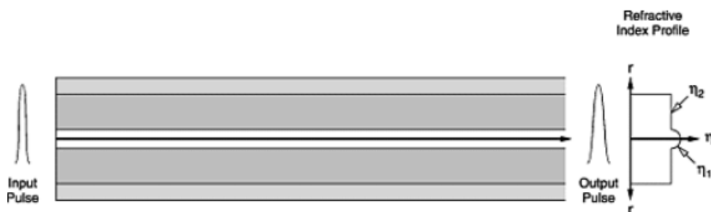
Gambar 3.9 Propagasi step indeks Single mode
